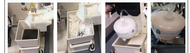
A coarse filter removes large pieces of wax/tissue; a fine filter (20 um pore size) removes smaller particles. Sections encounter only this doubly filtered water.
