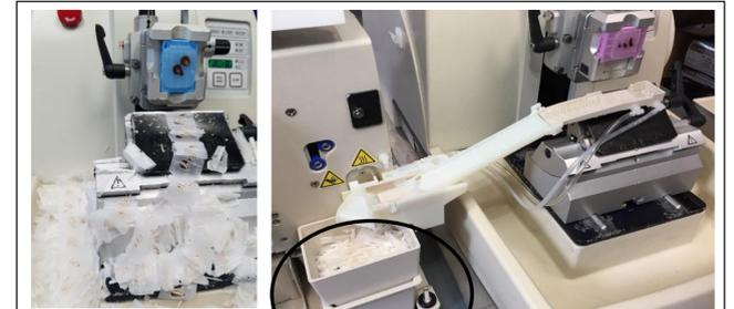
Paraffin can cause a mess in the lab, and can lead to falls. Aquaro ASM treats discarded sections (i.e. waste created by trimming/facing) much like “good” sections by floating them down the ramp and collecting them on a filter (instead of mounting them) for easy disposal.
